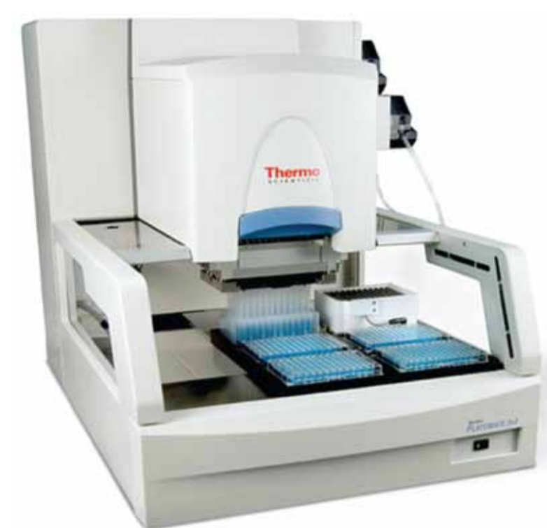
Automated fixation and staining by the Matrix Plate-Mate 2x2 pipetting robot
